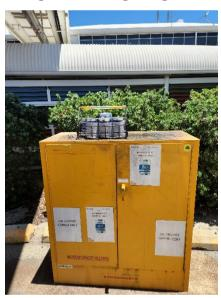
Aircraft engine oils and other similar substances must be stored in the provided oil storage cabinets and comply with storage and handling requirements of the Safety Data Sheet (SDS) and the Australian Standard AS 1940:2017 - The storage and handling of flammable and combustible liquids.
