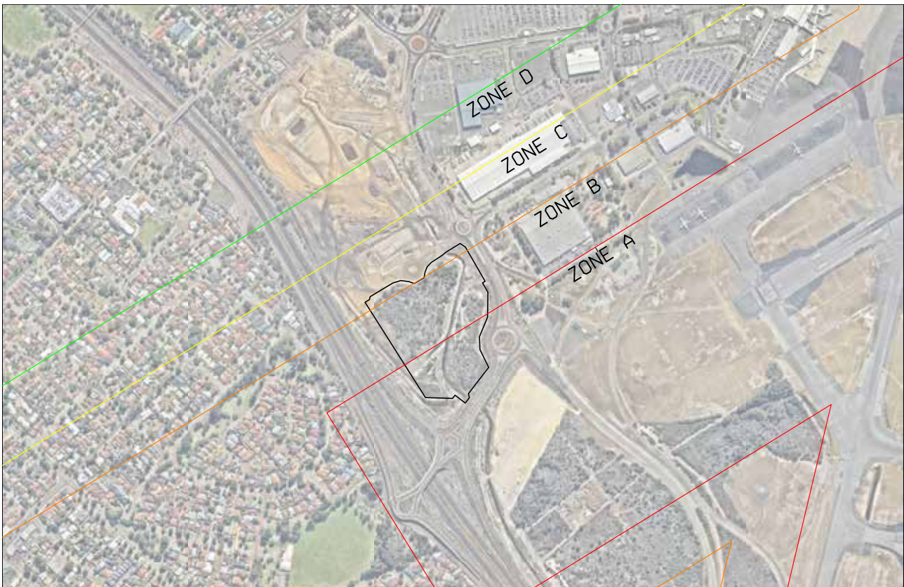
Figure 34 Lighting control zones
